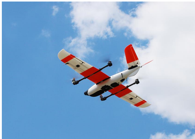
The Censys Sentero BVLOS aircraft in vertical climb just prior to forward-flight transition.
