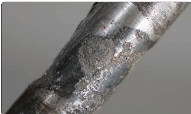
Figure 8-10. Dissimilar metal corrosion.
