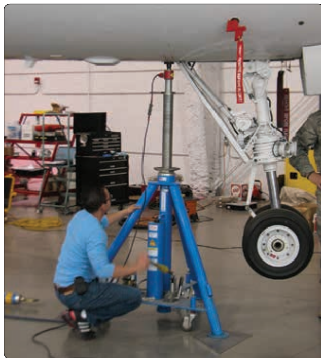
Figure 6-20. Airplane on jacks with load cells in use.
