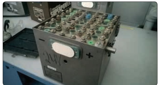
Figure 12-198. Nickel Cadmium aircraft battery.
