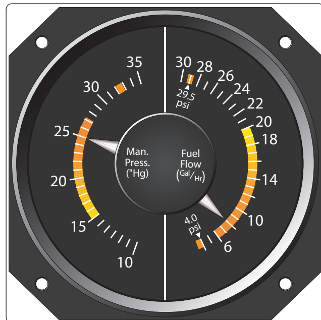
Figure 5-35. Manifold pressure gauge indicating absolute pressure.
