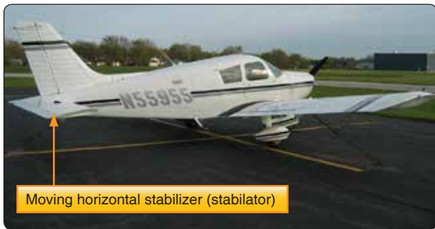
Figure 5-66. Moving horizontal stabilizer, known as a stabilator, on a Piper Cherokee Cruiser PA-28-140 provides pitch control.
