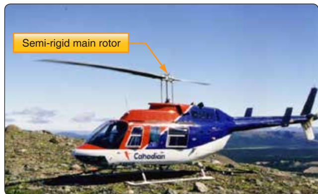
Figure 5-84. Bell Jet Ranger with semi-rigid main rotor.
