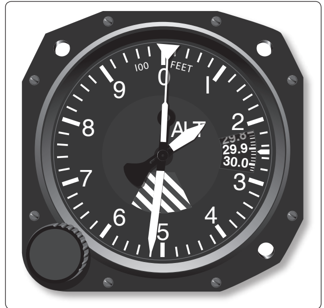
Figure 5-51. An airplane's altimeter is an aneroid barometer.
