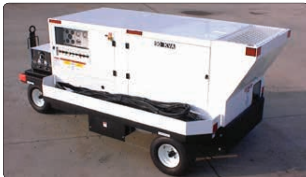
Figure 1-27. A mobile electrical power unit.
