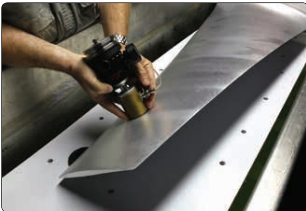
Figure 10-25. Ultrasonic inspection of a composite structure.
