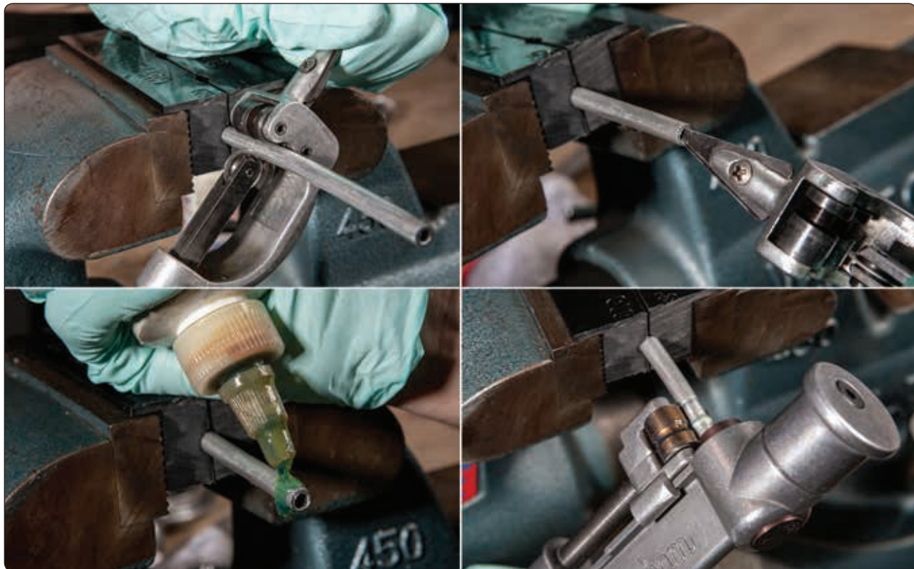
Figure 9-15. To use the hand beading tool, cut with tube cutter (1), deburr (2), oil (3), and revolve tool around tube while tightening handle (4).
