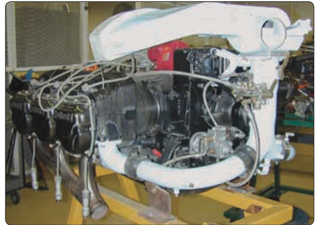
Figure 5-29. Aircraft piston engine cooled by convection.
