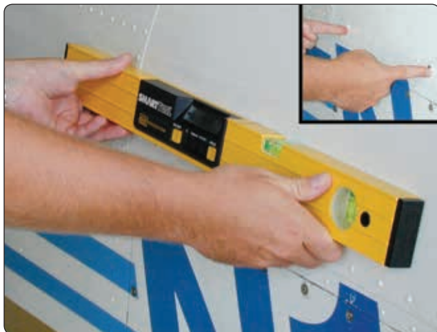
Figure 6-21. Spirit level being used on a Mooney M20.
