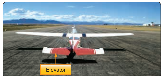
Figure 5-65. Elevator on a Cessna 182 provides pitch control.
