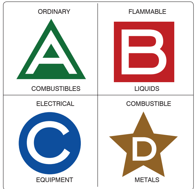
Figure 1-8. Identification of fire extinguisher type location.
