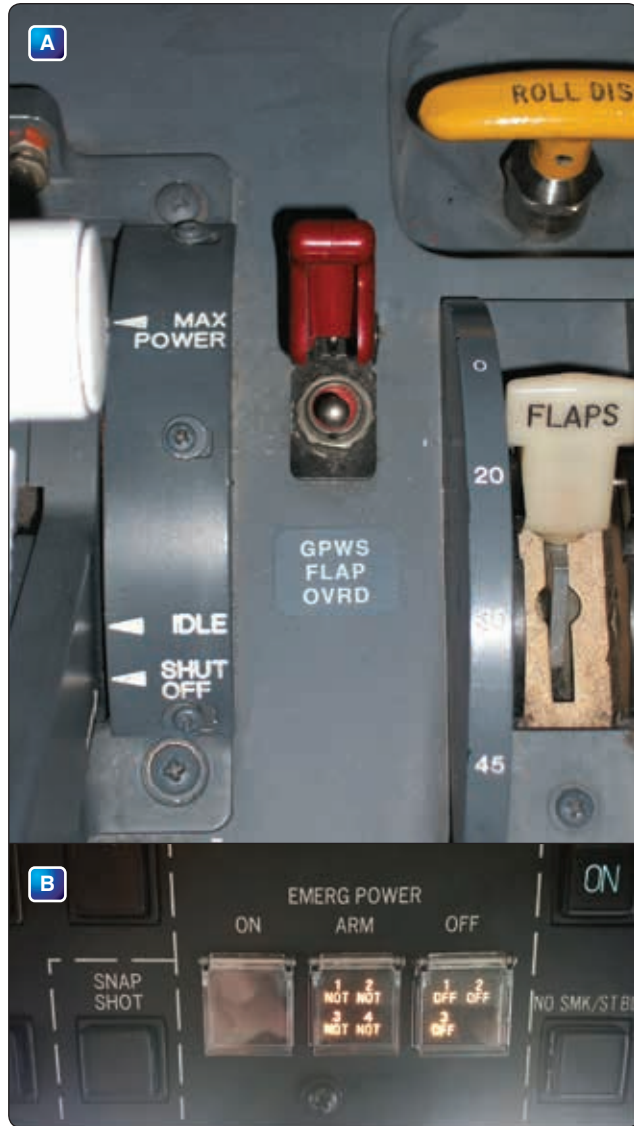
Figure 12-79. (A) Red guarded switch. (B) Push button switch with a guard.
