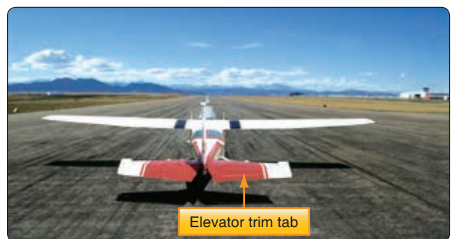
Figure 5-71. Elevator trim tab on a Cessna 182.
