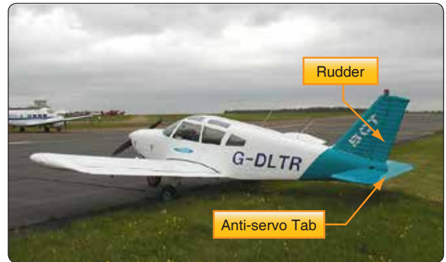
Figure 5-70. Rudder and anti-servo tab on a Piper Cherokee Arrow.
