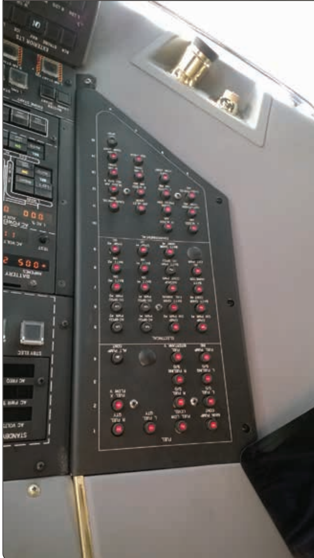
Figure 12-69. Circuit breaker assembly for aircraft electrical system.
