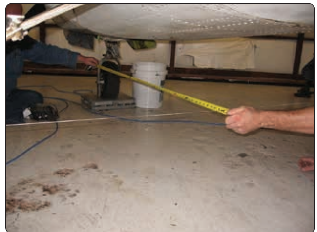
Figure 6-23. Measuring the nosewheel arm on an airplane.
