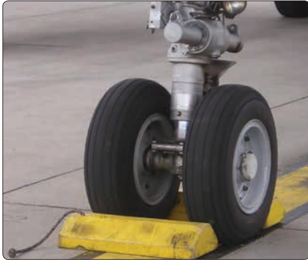
Figure 1-12. Wheels chocked fore and aft.
