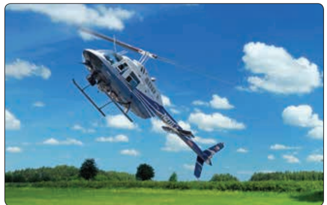
Figure 5-96. Bell Jet Ranger in final stage of autorotation.
