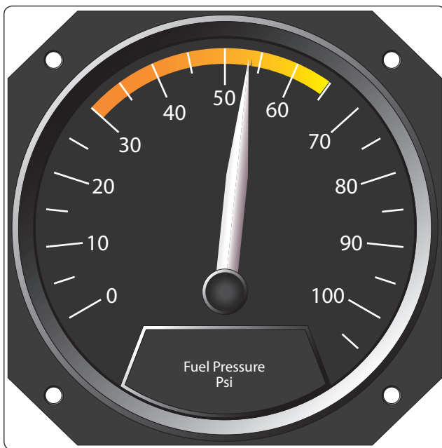
Figure 5-34. Psig read on a fuel pressure gauge.
