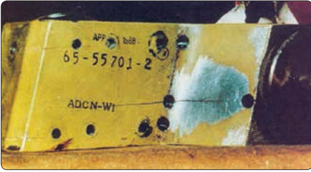
Figure 8-16. Stress corrosion cracking.
