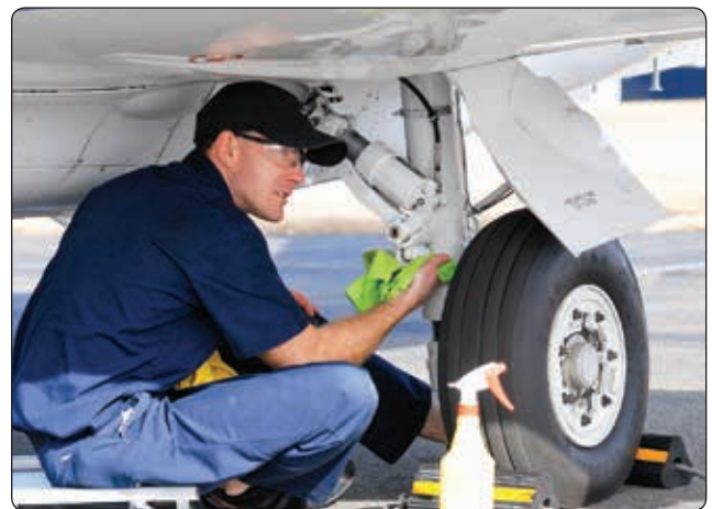
Figure 8-20. The landing gear area should be cleaned and inspected more frequently than other areas.
