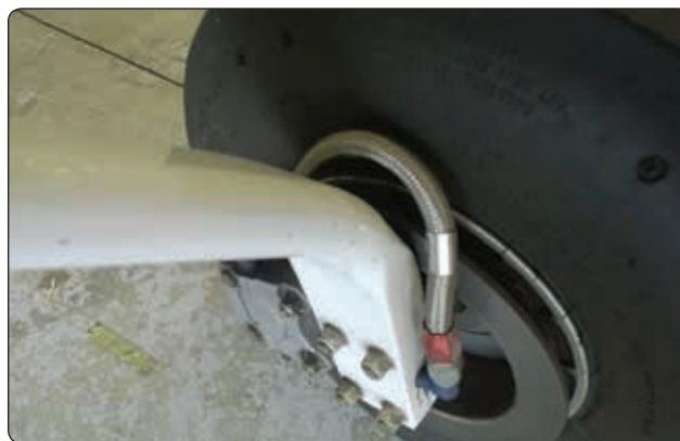
Figure 9-32. Flexible hose with stainless braid.
