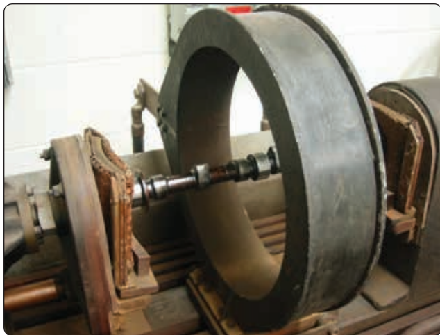
Figure 10-30. Longitudinal magnetization of camshaft (solenoid method).
